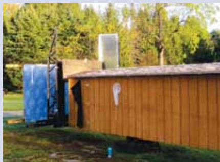
The tunnel – an apparatus for safely testing effectiveness of different materials and designs for deterring bird collisions. Photo: Christine Sheppard, ABC
